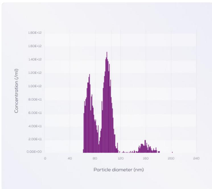
**Figure 2:** Size-based distribution of carboxylated polystyrene particles measured using the Exoid. The single-particle nature of TRPS measurements enables the three subpopulations in the sample to be resolved at a high level of resolution.
