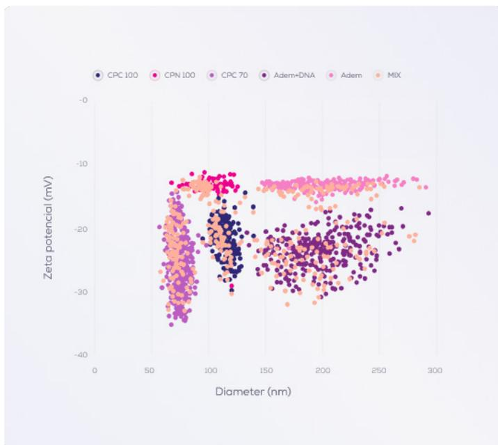
**Figure 4:** Zeta potential vs particle size of bare polystyrene particles (CPN100), carboxylated polystyrene particles (CPC70, CPC100), magnetic particles (Bio-Adembeads) and magnetic particles modified with DNA. The mix of five particle types closely resembles particle distribution when particle types are measured separately. Vogel et al. (2017). Sci Rep 7, 17479.
