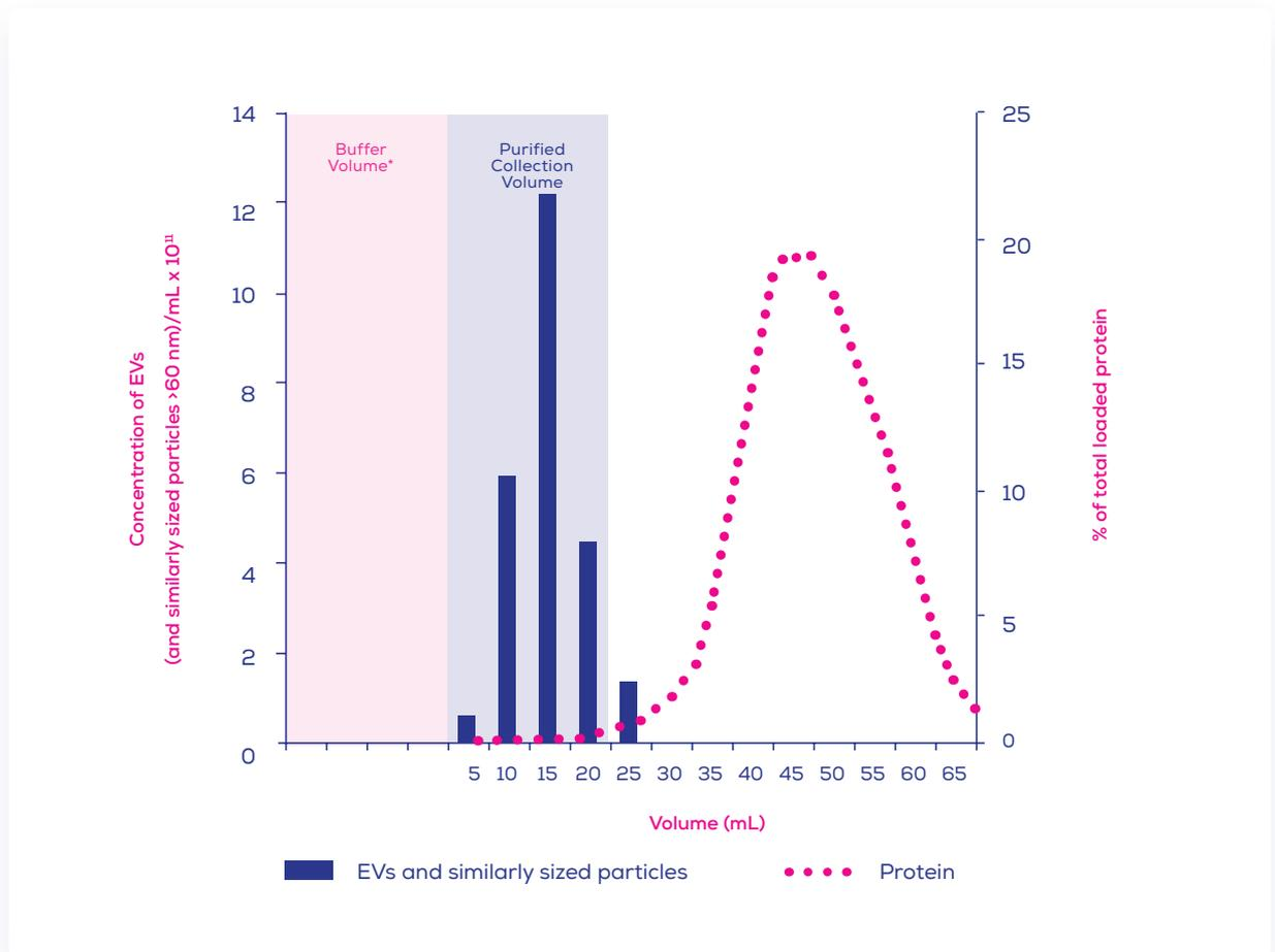
**Figure 2.** Typical elution profile for qEV10/35 nm Gen 2 columns with 10 mL of human plasma loaded; proteins elute at a later volume than extracellular vesicles and similarly sized particles >60 nm. EV concentration was measured using an Exoid and protein levels by bicinchoninic acid (BCA) assay. \*Recommended buffer volume values vary for qEV10/35 nm and qEV10/70 nm columns: refer to your qEV User Manual for guidance.
