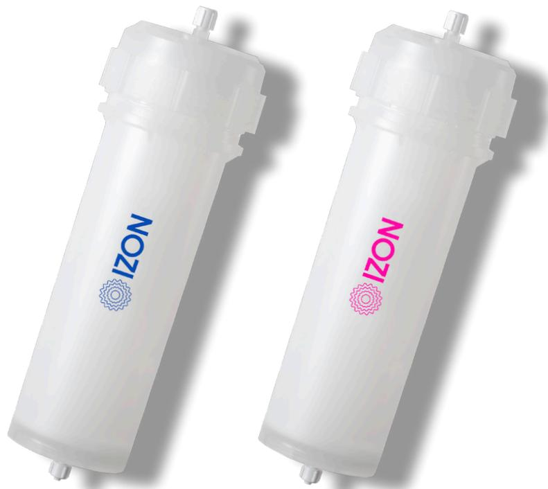
**Figure 1.** The qEV100 Gen 2, capable of running 100 mL samples. Like all columns in the qEV range, qEV100 Gen 2 columns are available in two types: the 35 nm Series (left, provides optimal recovery of particles in the range of 35-350 nm) and the 70 nm Series (right, provides optimal recovery of particles in the range of 70-1000 nm).
