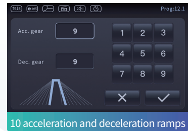
10 acceleration and deceleration ramps
