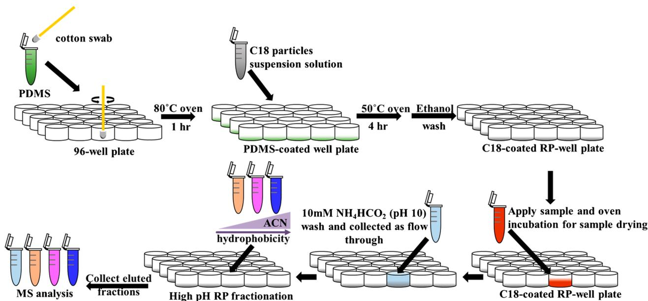
**Fig. 1** Schematic representation of the functionalized RP-well plate fabrication and peptide fractionation procedures
